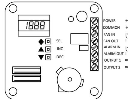
Recommended cable type is 14-24 AWG shielded twisted pair. For runs over 200 feet use a minimum of 22 AWG.
